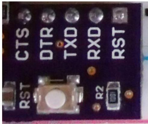
To use the USB to UART just connect to the pins on the breadboard and you are set. DTR has a 100nf ceramic cap in series for all those who want to program an Arduino.
