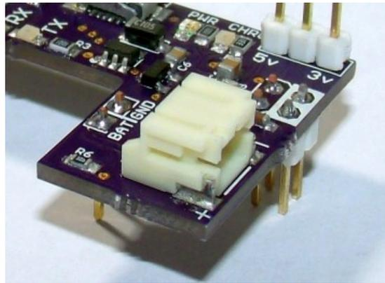
Uses the widely known and trusted MCP73831 for lipo charging. These ICs are so popular and tested so much that it almost guarantees your battery will be charged safely. The same charging circuit is used by other suppliers of similar circuits. What makes mines special is the ability to still supply power to circuit while charging, without crossing the voltage. Has a option for 100mA or 500mA charging on bottom. (Solder Jumper)
